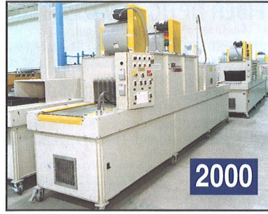
2000 ITW-BGK 92.2-KW 6-ZONE CONVEYORIZED INFRARED SILK SCREEN CURING OVEN
