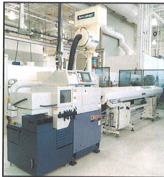
1 OF 4 CITIZEN MODEL B-12 CINCOM SINGLE-SPINDLE CNC SWISS-TYPE SCREW MACHINES
