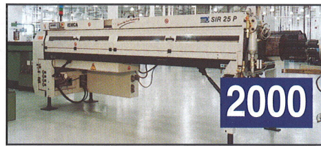
IEMCA MODEL SIR25/38P AUTOMATIC MAGAZINE-TYPE MULTI-SPINDLE BAR FEED
