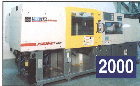
1 OF 4 CINCINNATI-MILACRON ROBO 110I-97 RECIPROCATING SCREW PLASTIC INJECTION MOLDING MACHINES
