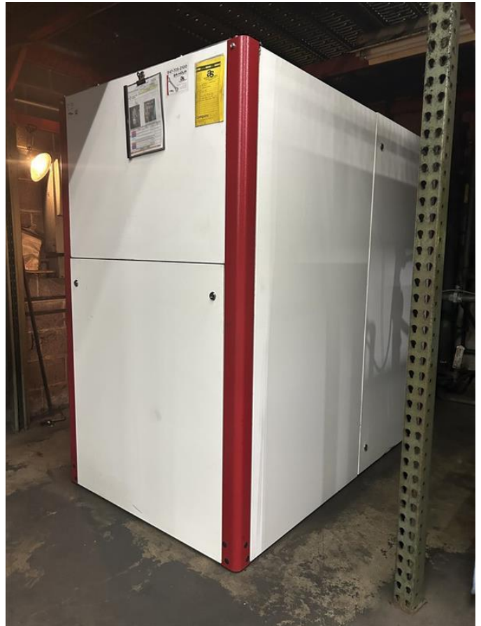
#44747 GARDNER DENVER LRS55-75F ROTARY SCREW AIR COMPRESSOR 75 hp, 6857.6 Hours
