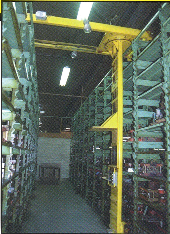
2,000 LB. ELECTRIC SWIVELING DIE LIFT
