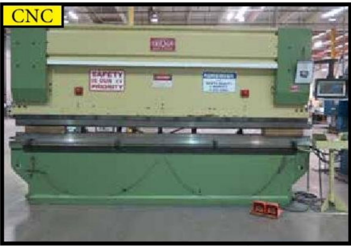
CNC Chicago HPB11040 120 Ton x 13' CNC Hydraulic Press Brake w/ SB-230- Controls
