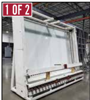
Single Glass Inspection Lighted Station
