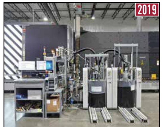
LISEC Insulated Glass Assembly Line
