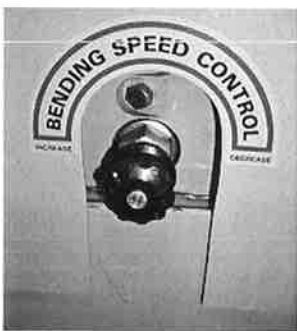
Figure 5.6-3: Variable Ram Speed Control
