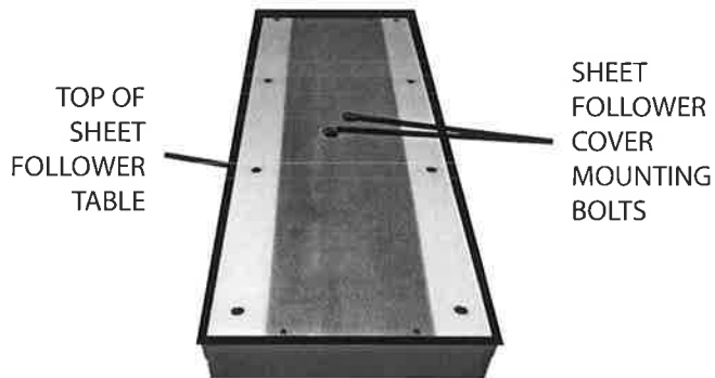
Figure 9.4-1: Removing Cover Mounting Bolts from the Top of the SF Table
