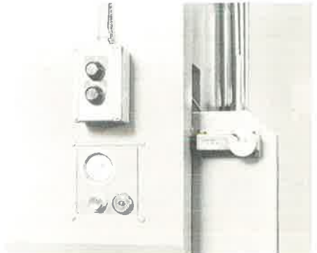
FRONT OPERATED STROKE CONTROL WITH DIGITAL COUNTER TONNAGE INDICATOR AND CONTROL.
