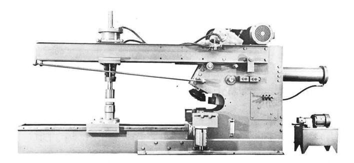
This machine will flange all flat heads from 20" to 12' diameter. Attachments available for flanging dished heads from 30" to 12'. Offset rolls available for this machine. Shipping weight 6,000 lbs. Motor 7½ H.P., 1800 R.P.M.
