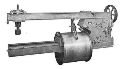
No. 3—¼" capacity Blue Valley Flanging Machine for flanging flat heads only from 19" to 12'. Equipped with two upper flat head rolls; pneumatic center holddown; 5 H.P. motor, 1800 R.P.M., 220/440/3/60; and with tooling and attachments for flanging tubes from 24" to 60" diameters x 60" long, in all thicknesses up to ¼"; less the foundation, base or pit.
