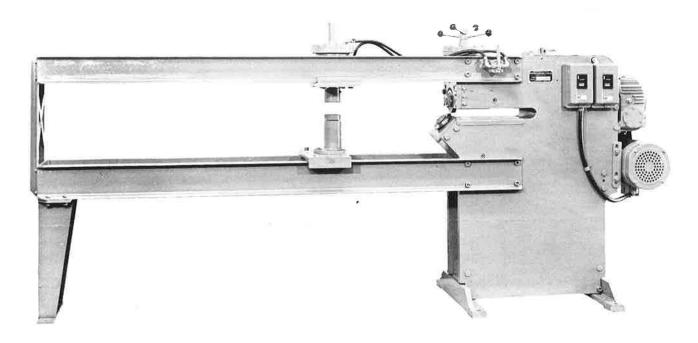
This machine will shear from 12" to 12'3" dia. at speed of 40 feet per minute. Motor is 3 HP, 1800 RPM. Weight 1,800 lbs.
