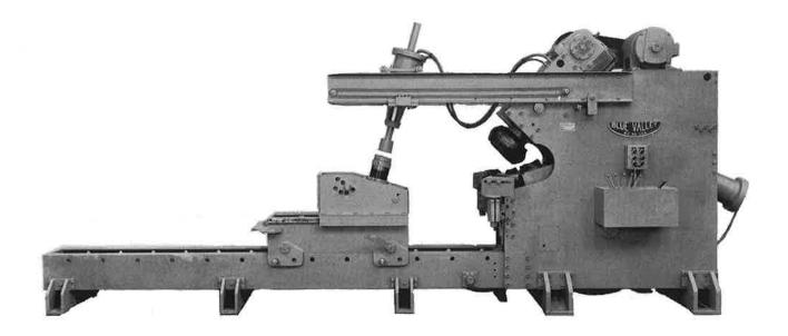
This machine will flange dished heads from 48" to 18'. Shipping weight is 20,000 lbs. Motor is 50 HP, 1800 RPM.
