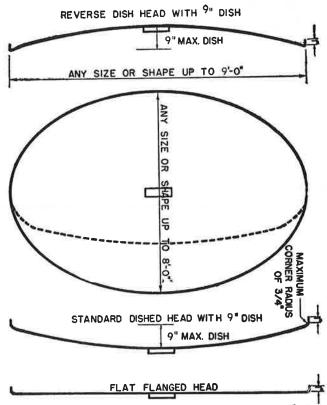
Above is shown a cut of the different type and shape heads than can be sheared and flanged.
