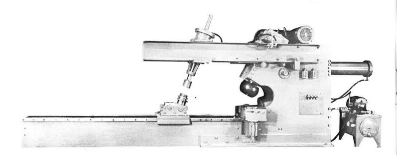
This machine will flange all flat heads from 24" to 20' diameter. Attachments available for flanging dished heads from 36" to 13'. Shipping weight 9,500 lbs. Motor 10 H.P., 1800 R.P.M.
