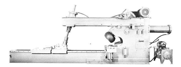
This machine will flange all flat heads from 28" to 20'. Attachments available for flanging dished heads from 36" to 13'. Shipping weight 11,500 lbs. Motor 20 H.P., 1800 RPM
