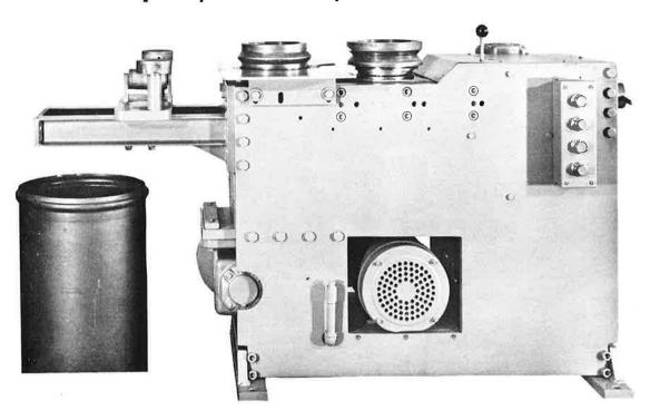
For offsetting tank tubes from 12" to 36". Weight of machine is 2,000 lbs. Motor is 5 HP, 1800 RPM. Machine equipped with hydraulic power unit with 1 HP motor.
