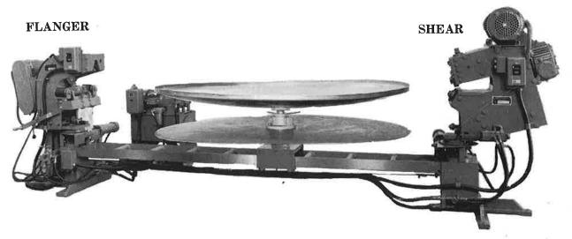
Blue Valley Elliptical Head Shear and Flanging Machine which operates from the same controls. Shears the head to size and shape before flanging it from the same template, without removing it from the machine. Weight of machine, 3,400 lbs.
