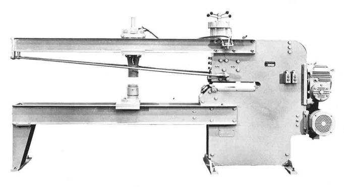
This machine will shear from 15" to 12'3" dia. at speed of 40 feet per minute. Motor is 10 HP, 1800 RPM. Weight 4,000 lbs.
