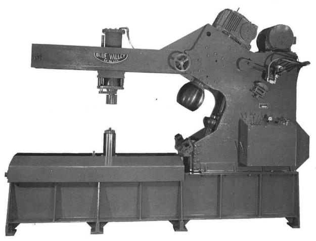
Developed for flanging 2 to 1 ratio dished heads as well as the standard dished heads.
