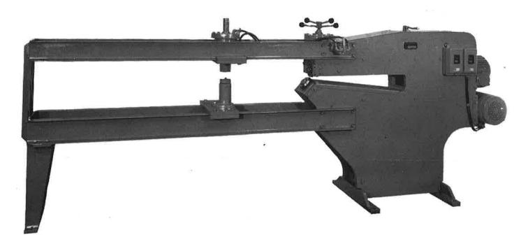
This machine will shear from 12" to 12'3" dia. at speed of 40 feet per minute. Motor is 3 HP, 1800 RPM. Weight 3,000 lbs. 30" throat depth.
