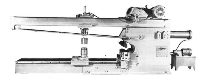
This machine will flange all flat heads from 19" to 12' diameter without any hole in the center of the head. This No. 3 machine is for flat heads only and is not furnished with dished head attachments. Offset rolls are available for this machine. Shipping weight 3,400 lbs. Motor 5 H.P., 1800 R.P.M.
