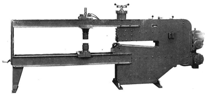
The machine will shear from 15" to 12'3" dia. at speed of 40 feet per minute. Motor is 10 HP, 1800 RPM. Weight 5,500 lbs.
