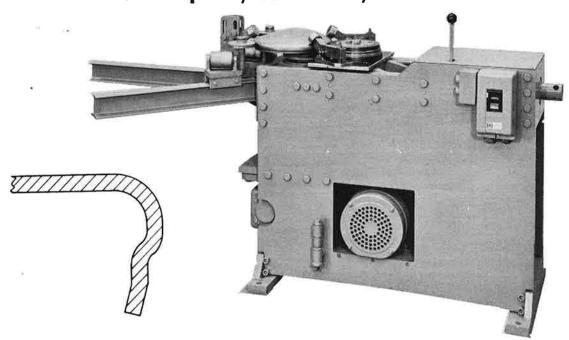
For offsetting tank heads from 12" to 36". Weight of machine is 2,000 lbs. Motor is 5 HP, 1800 RPM. Machine equipped with hydraulic power unit with 1 HP motor.
