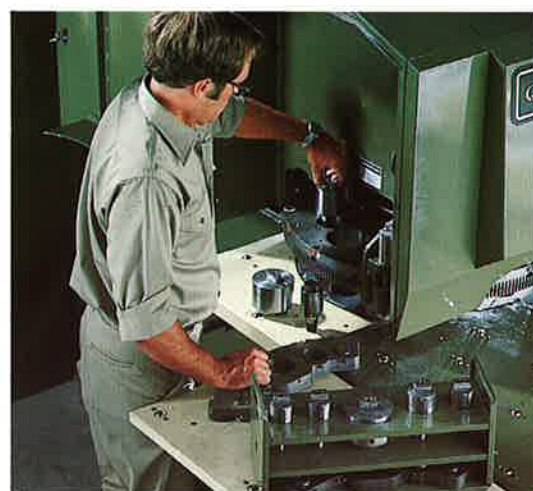
Operator then removes five punch holders and places them in empty storage rack.
