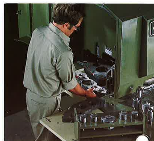
Operator takes fresh, pre-programmed die cartridge from previously-loaded storage rack and inserts it into lower turret.
