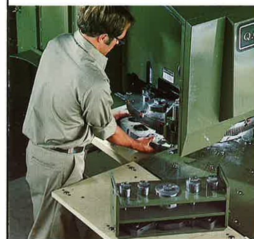
As tool change door opens, table segment in front of lower turret drops to change position. Die cartridge is then removed from lower turret.
