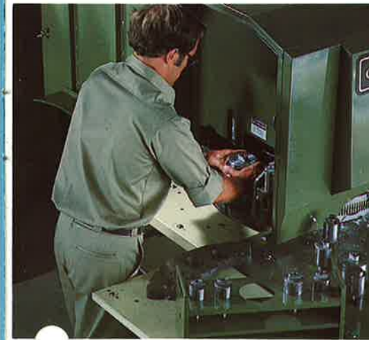
Punch holders, also previously loaded, are removed from storage rack and inserted into upper turret.
