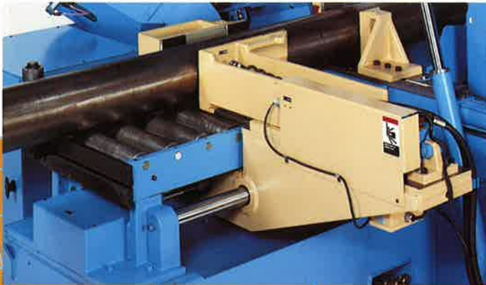
Automatic material feed is handled by a unique, space-saving underslung C section design. The heavy-duty roller conveyor is integrated with the saw frame, eliminating adjustments, simplifying installation, and reducing friction when cutting forged or crooked bars.
