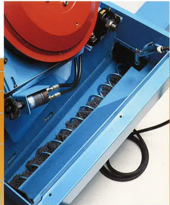
Chips are removed from the blade tooth gullets by a hydraulically driven, adjustable band brush and deposited into a powerful screw auger conveyor.
