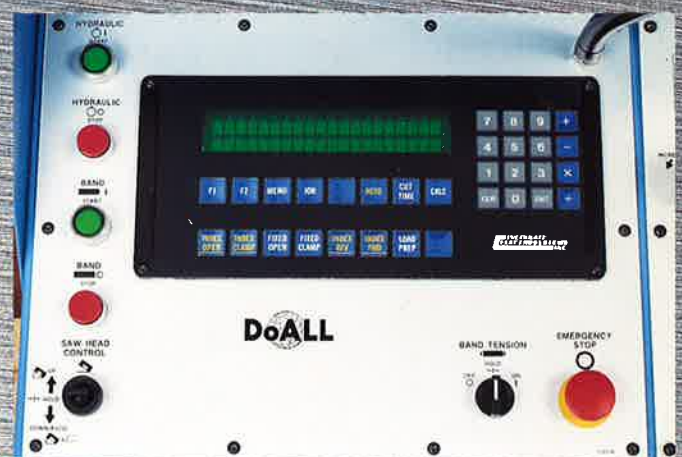
NC Control is conveniently located and features two line alpha/numeric-inch or millimeter display with prompting messages.
