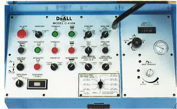
All control functions are conveniently located at the front of the machine, including hydraulic feed, digital index length readout, and band speed changes.
