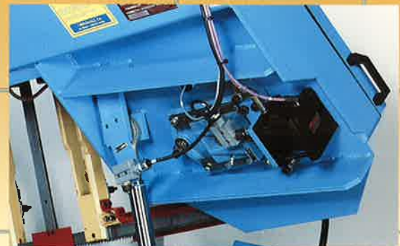
Hydraulic cylinder is activated at operator control console to engage factory set band tension.
