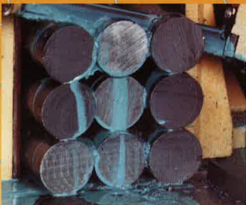
Optional hydraulic nesting fixture holds stacked work firmly for economical sawing of multiple workpieces.
