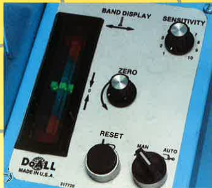
Band twist monitor (optional) constantly checks squareness of cut and automatically shuts band off if operator-set tolerances are exceeded.
