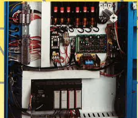
Electrical components are housed in oil-tight enclosure directly below operator's station. All wires are numbered for easy maintenance.
