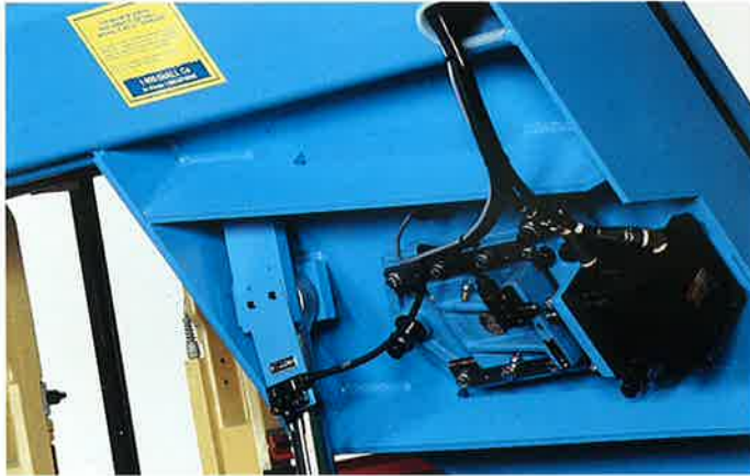
Band tension is factory set to 30,000 psi (207 MPa) for maximum blade stiffness. Hydraulic cylinder acting as idler wheel slide assembly is controlled by operator. Machine stops automatically if band breaks.
