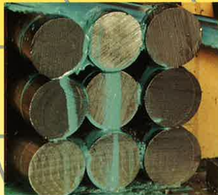
Nesting fixture (optional) holds stacked workpieces firmly for economical sawing of multiple pieces.
