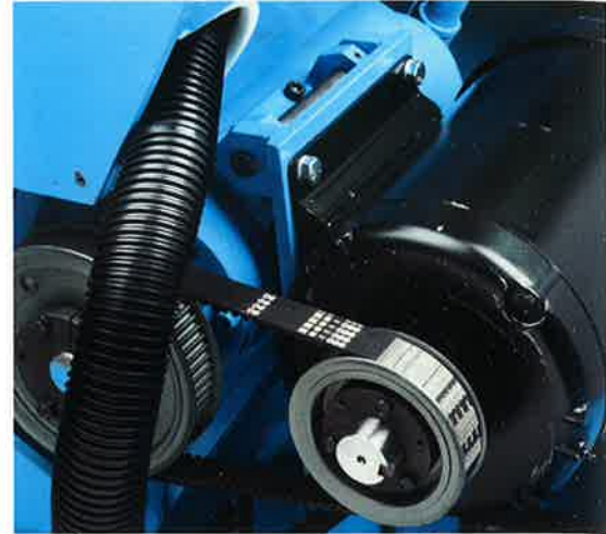
Simple, powerful bandwheel drive consists of a 10 hp (7.5 kw) electric motor coupled to an energy efficient worm gear box.
