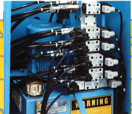
Ten-gallon (37 liter) hydraulic system with 6 gpm (23 lpm) energy efficient, pressure-compensated pump is located at rear of machine. Single manifold includes all solenoids for easy maintenance.
