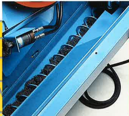
Chips are removed from blade tooth gullets by hydraulically driven, adjustable band brush and deposited into powerful screw-type auger conveyor for disposal.
