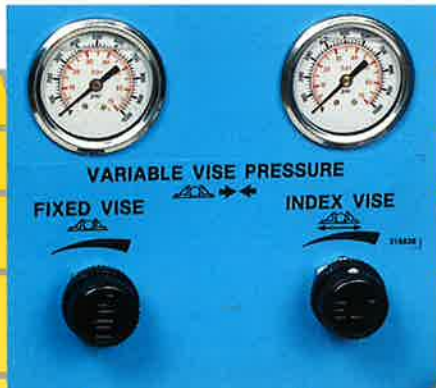
Variable pressure adjustment of both fixed and index vises permits the automatic sawing of tubing and other hollow, thin-wall materials without crushing or distortion.
