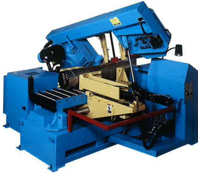
Outboard hydraulic cylinder provides wide stance 3-point head support to minimize vibration during sawing.
