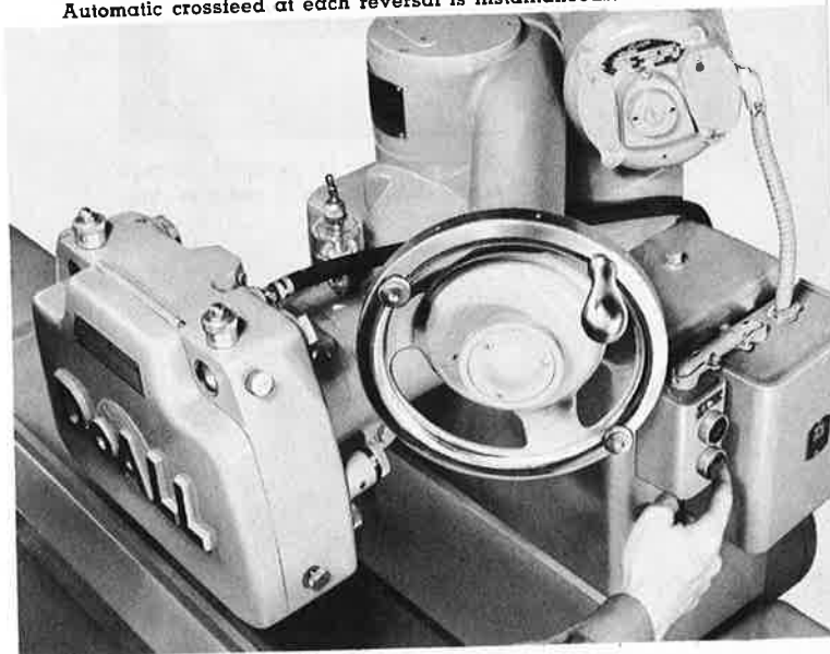
Power Vertical Adjustment — For rapid positioning of wheel heads. Relieves operator fatigue and speeds production. (Extra charge on D6 Models.)
