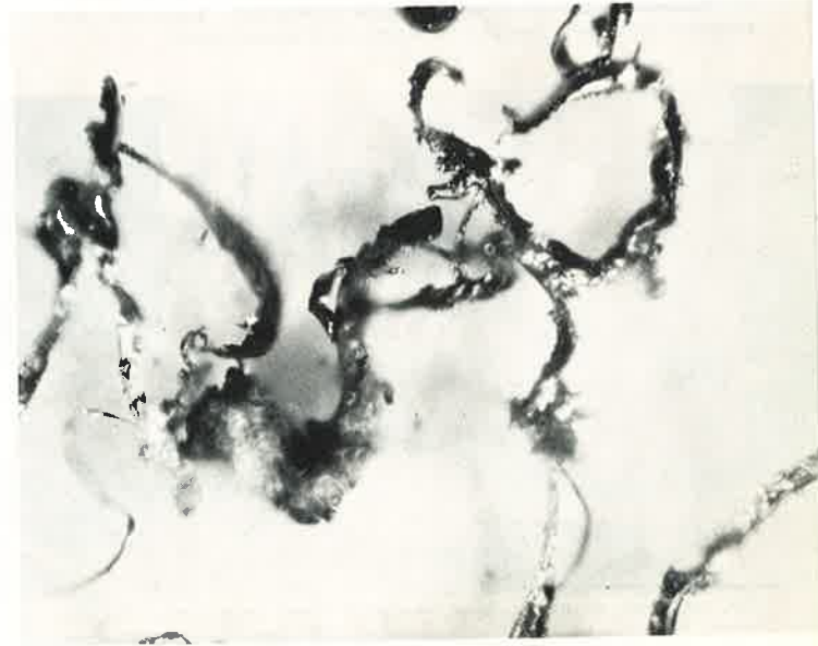
"COOL GRINDING" — Complete absence of globules and presence of long chips indicate heat absorption by coolant, better finish and accuracy.
