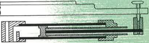
Floating Piston Rod —Exclusive construction feature prevents piston rod, that connects table to hydraulic cylinder, from touching cylinder. Temperature changes or cylinder misalignment cannot cause shifting of table. Table support ways on top of saddle are extra long.
