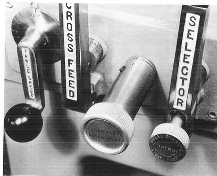
Variable Wheel-Dressing Speeds — The hydraulic wheel dressing feed is provided with infinitely variable speeds for coarse or fine dressing. This feature is also used for work-positioning, cylindrical grinding, broach grinding and similar work.
