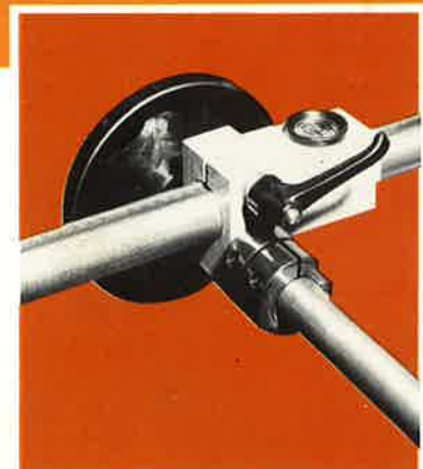
Magnifying dimensional indicator on rack and pinion back gauge.
