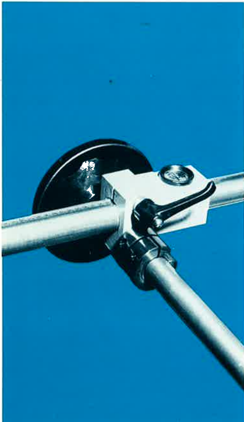
Magnifying Dimensional Indicator on Rack and Pinion back gauge.
