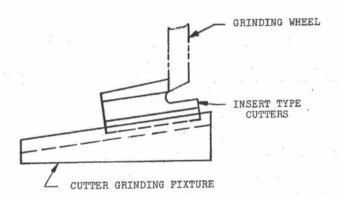
The Mitts & Merrill Cutter Grinding Fixture allows Mitts & Merrill keyseater users to save time and money by enabling them to grind cutter inserts in-plant easily and precisely on any universal grinder.
