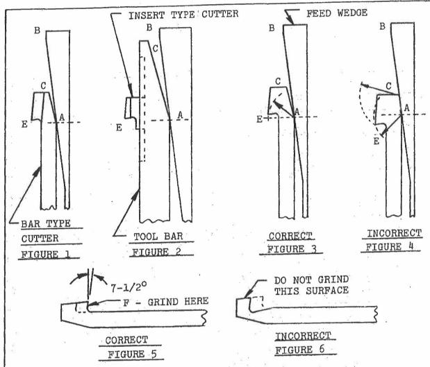
Figure 1 shows the style of cutters which are furnished with posts up to 1-1/4" diameter. Figure 2 shows the style generally furnished with 1-1/2"
