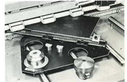
Gauge Clamps for shearing to punch marks or scribed line.
